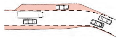
Figure 8.19 Gradual widening of the carriageway to create on-street spaces, with running carriageway checked using vehicle tracking.
