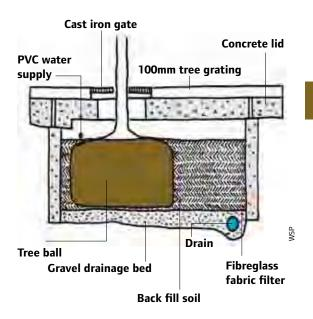
Figure 11.4 Typical tree pit detail.
