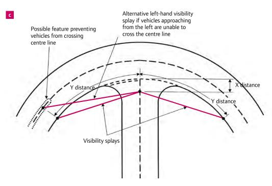
Figure 7.18 Measurement of junction visibility splays (a) on a straight road, (b) and (c) on bends.
