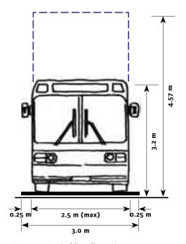
Figure 6.16 Typical bus dimensions
