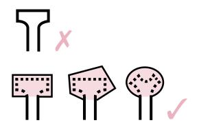
Figure 7.24 Different turning spaces and usable turning heads.
