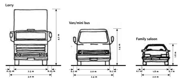
Figure 6.18 Private and commercial motor-vehicles - typical dimensions.
