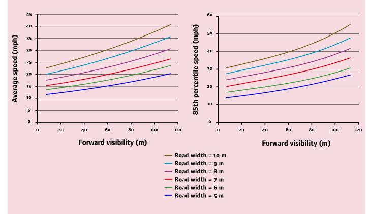
Figure 7.16 Correlation between visibility and carriageway width and vehicle speeds (a) average speeds and (b) 85th percentile speeds. These graphs can be used to give an indication of the speed at which traffic will travel for a given carriageway width/forward visibility combination.
