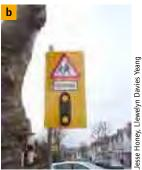
Figure 9.1 (a) Sign clutter in residential areas; (b) the yellow backing board adds clutter and its use with the flashing amber lights is counter-productive. In addition, the sign post should not protrude above the sign.
