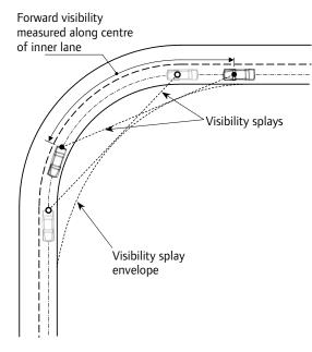
Figure 7.19 Measurement of forward visibility.
