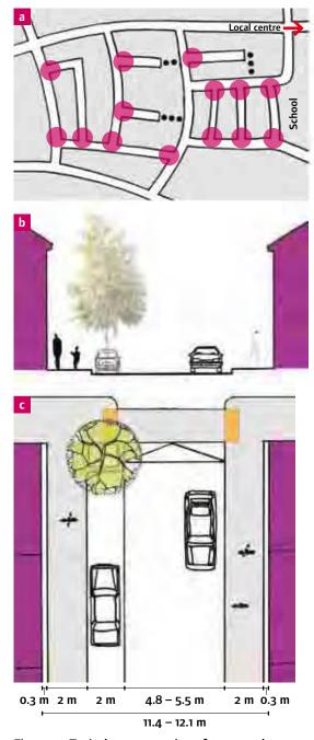
Figure 7.2 Typical representation of a street character type. This example shows the detail for minor side street junctions. Key plan (a) shows the locations, (b) is a cross-section and (c) the plan.
