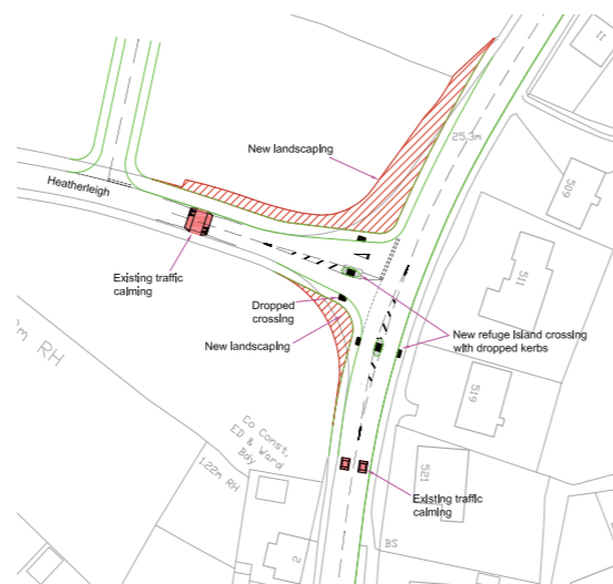
Proposed junction improvements along Heatherleigh
