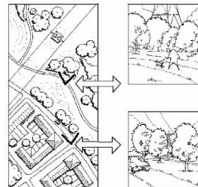
Image showing how public open space can screen views to pylon structures
