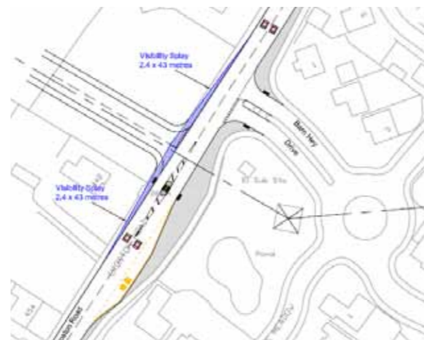
Proposed junction alterations at Croston Road
